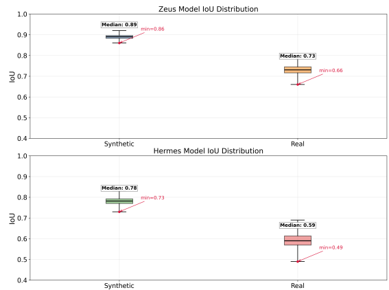
Fig. 5: IoU distribution for Zeus and Hermes models on synthetic and real data.
