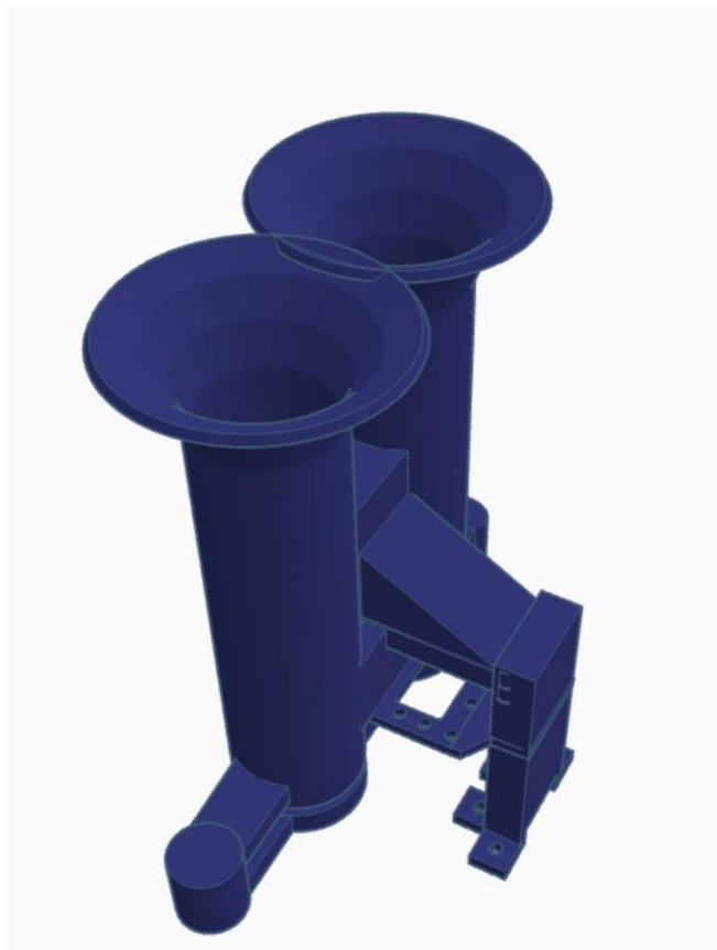
Fig. 4. This is a screenshot of the CAD design for the drum container.
